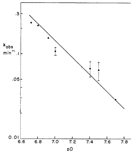
Figure 2. Rate of decarboxylation of N-carboxy-2-imidazolidone as a function of pD at 25°. Vertical bars represent the average deviation in cases where more than one determination was made. The slope of the line is 1.0.
