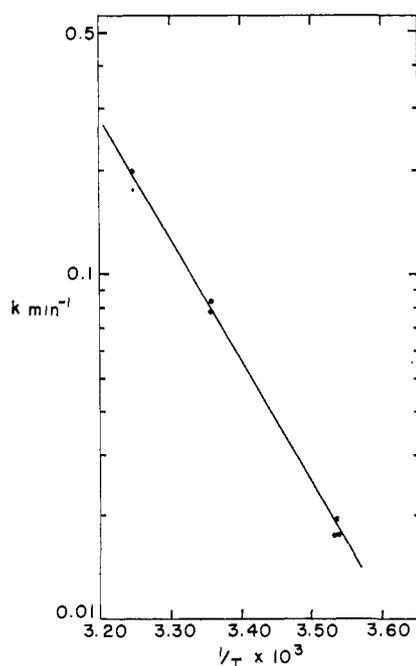
Figure 3. Arrhenius plot of the rate of decarboxylation of N-carboxy-2-imidazolidone at pD 7.4.
